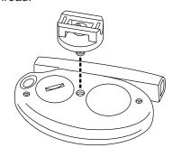
Secure to handlebar or strut using Velcro® strap. Fits bars <sup>3</sup>/<sub>4</sub>" to 1<sup>1</sup>/<sub>2</sub>" in diameter (19 to 38 mm).
