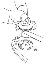
**2. Attach Mounting Bracket.** Attach mounting bracket to tripod thread.
