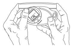
**Measure Wind Speed.** Point front of wind barrel into wind to measure positive (+) wind sped or headwind. Point rear of wind barrel into wind to measure negative (-) wind speed or tailwind.
